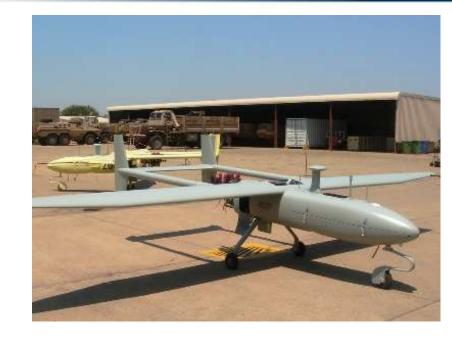
Operational range is 250 km limited by ELOS (Electronic Line Of Sight) to the ground control unit due to onboard directional antenna
