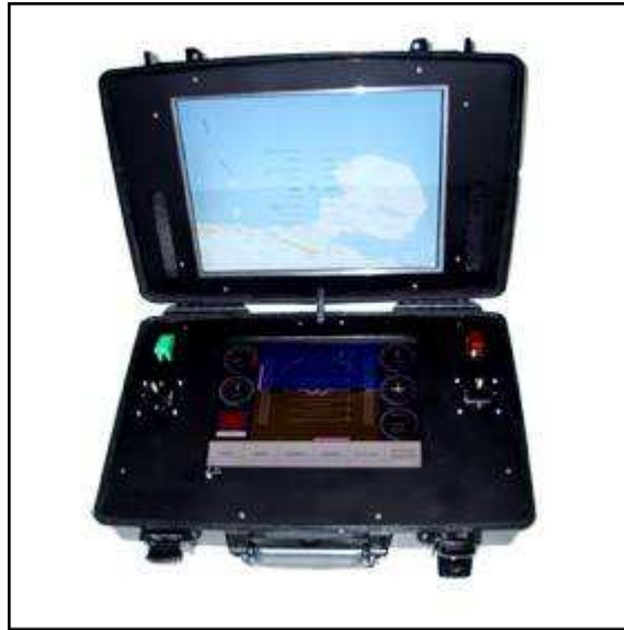
Figure 10: Typical small UAS Ground Station
