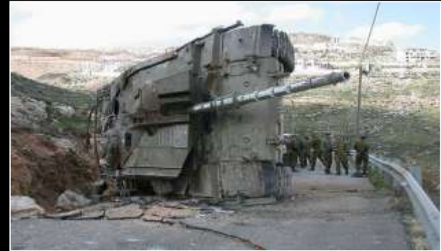
Effect of culvert IED on IDF Merkava MBT
