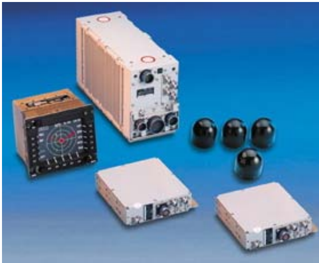
Figure 36: A typical RWR (left) and LWR (right) ESM system.
