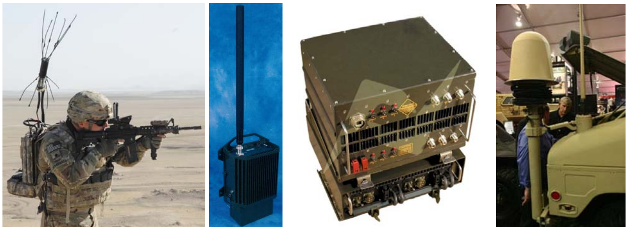
Figure 50: Man portable and vehicle mountable RF IED Jammer [SNC].
