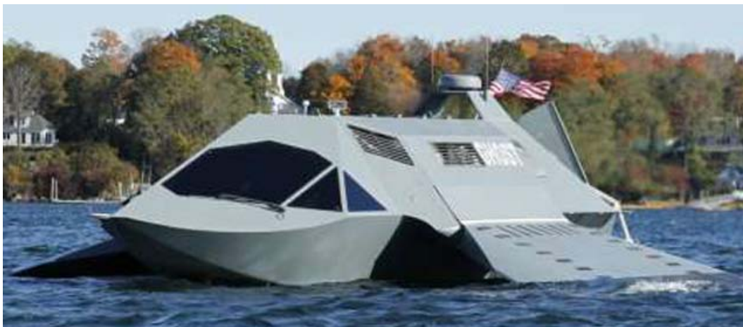
Figure 44: Hull design to reduce both the RCS as well as the wake signature.
