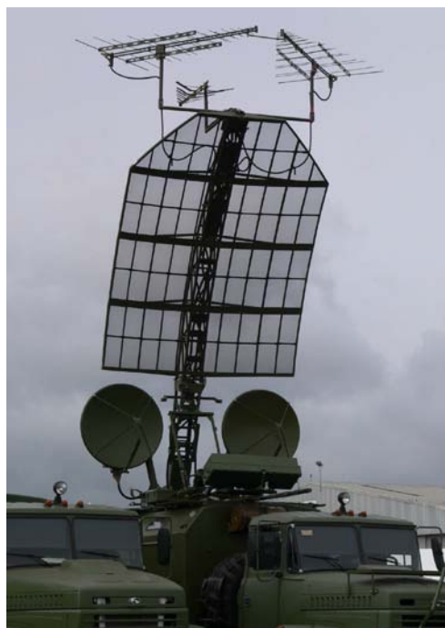
Figure 38: The Russian Kolchuga ELINT system. Four of these systems can be networked together to enable geo-location.
