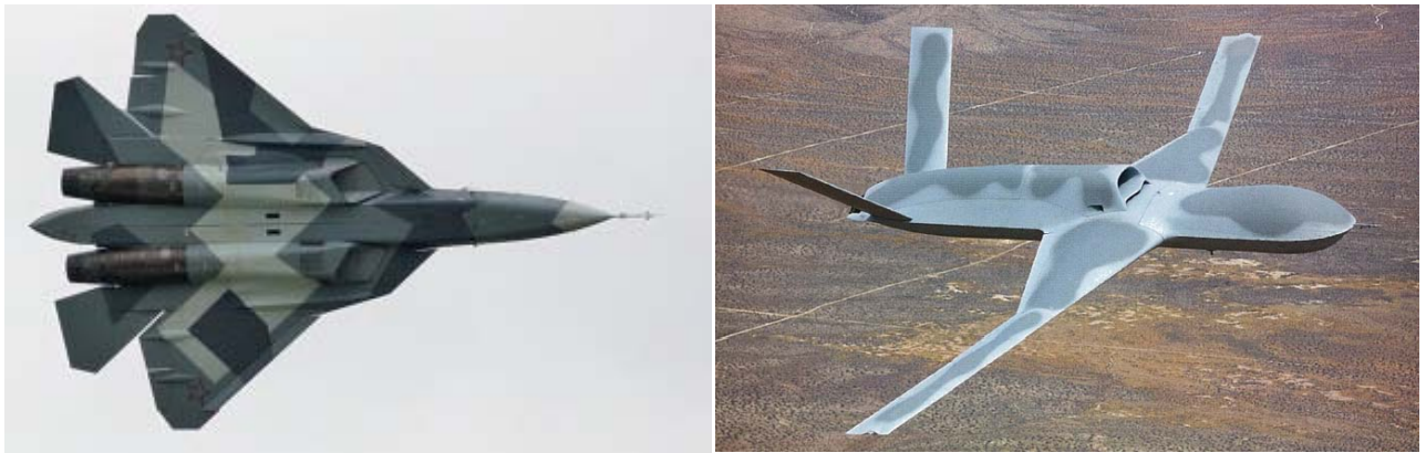
Figure 45: Russian SU-T 50 (left) and the new Predator UAV (right) – examples of low Radar Cross Section aircraft.
