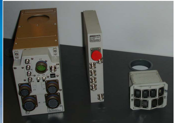
Figure 36: A typical RWR (left) and LWR (right) ESM system.
