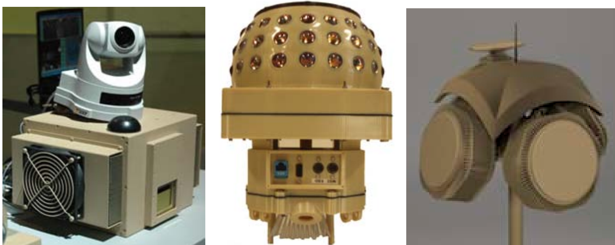
Figure 47: Apache helicopter's WeaponWatch sector (left), ShotSense3D Shortwave Infrared 360 deg (middle), Rada pulse Doppler radar HFI system (right)
