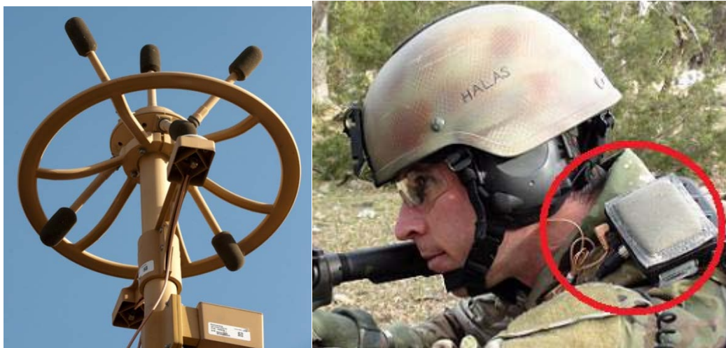
Figure 46: Boomerang acoustic (left), Soldier-Wearable Acoustic Targeting System (SWATS) (right).
