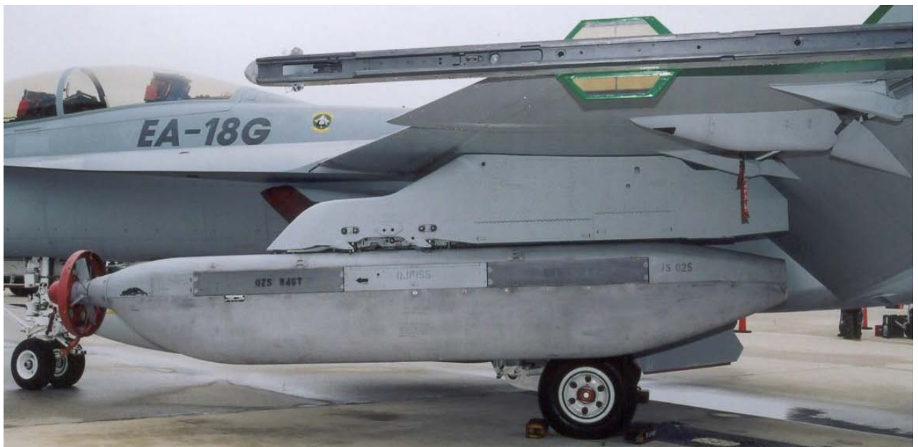
Figure 27: The Next Generation Jammer is scheduled to replace the legacy ALQ-99 jamming pod (shown here on an f-18 Growler).
