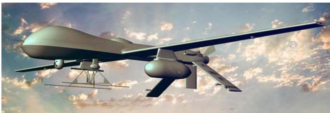
Figure 30: General Atomics MQ-9 UAV with jamming pod.
