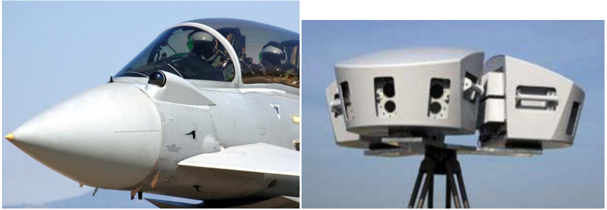
Figure 25: Examples of anIRST system on a fighter aircraft (left) and of the Thales Gatekeeper surveillance system (right).
