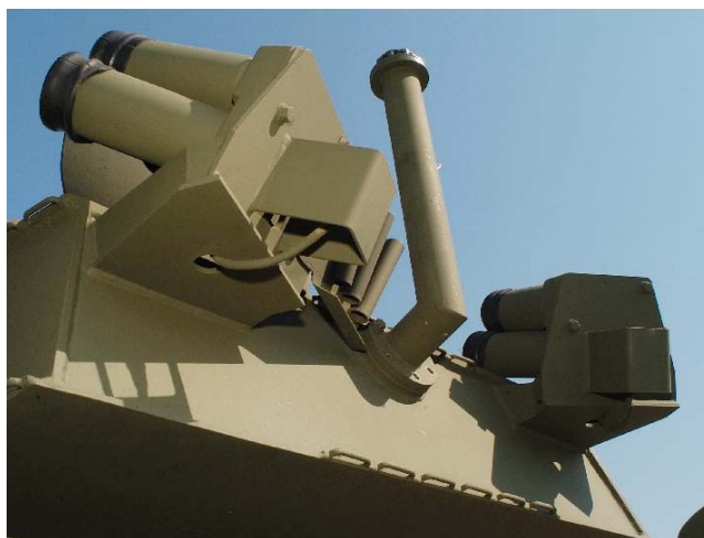
Figure 35: LWR fitted to an Amphibious Assault Vehicle (AAV) – integrated to the smoke launchers.
