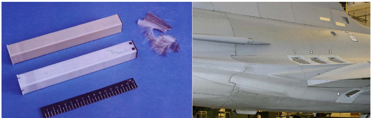
Figure 32: A typical airborne chaff cartridge & chaff (left), and the Gripen's chaff/flare dispensers (1 to 4) shown on the right.
