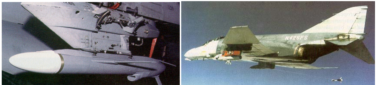
Figure 33: A Miniature Air-Launched Decoy (MALD) on an USAF F-18 (left), with an AN/ALE-55 Fibre-Optic Towed Decoy (FOTD) being launched from an USN F-4 (right).
