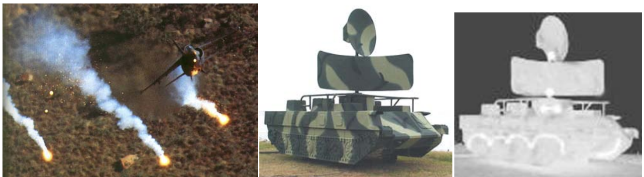
Figure 34: Mirage dispensing IR Flares (left) and a visual decoy with IR properties (right).
