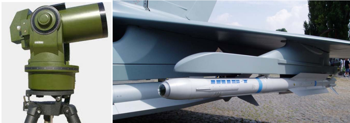
Figure 22 Luckyo 2.5 GBs laser communications link (left) and IRIS-T imaging IR missile (right).
