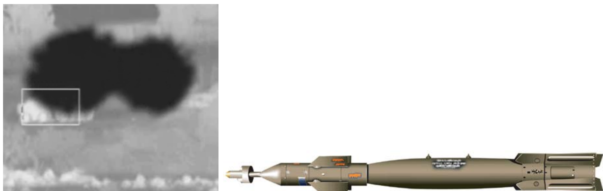
Figure 23: An Infrared image of smoke in the process of obscuring an armoured vehicle (left) against a Paveway II Laser Guided Bomb attack (right).
