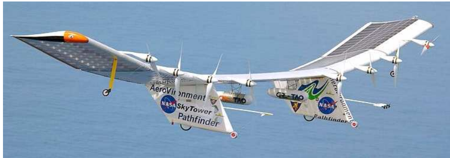
Figure 20: Pathfinder Plus UAV carrying Sky Tower Communication Relay Systems
